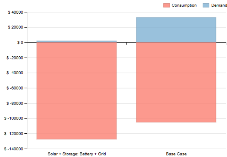
Figure 7. Comparison of utility bill components between the hybrid and base case systems
