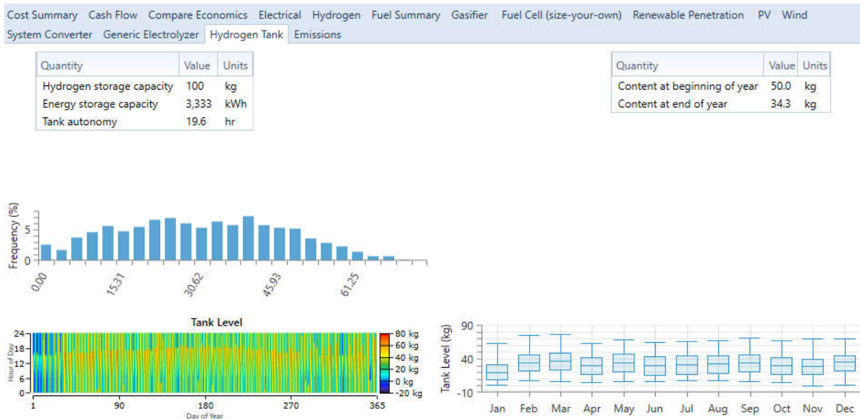
Figure 14. Hydrogen storage tank performance and utilization
